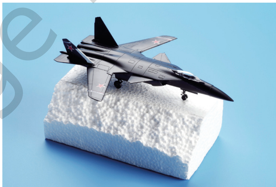
FIGURE 15.4.11 A model plane made of rigid polystyrene sitting on a block of foamed polystyrene.
